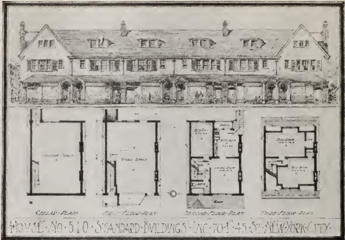
Plan Showing Tenement Type of Building for Workingmen. Example of One of Fifty Plans Submitted
